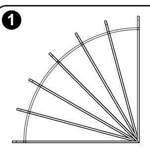
Before starting the construction it is a good idea to lay the rafters out on the ground and make sure that they all line up, and for the positioning of the posts.
