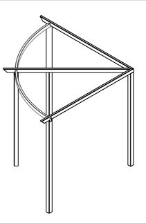
Place Rafter 4 so that the notch overlaps the join between the two arc rafters and sits on the un notched post central, between the other rafters.
