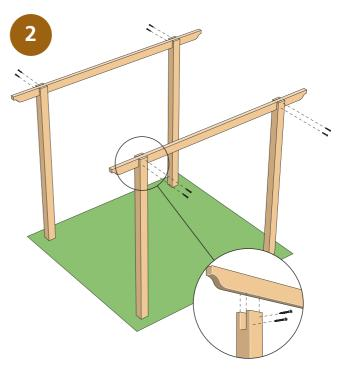
Drop a rafter into the Metclips and adjust to ensure that the overhang at each side is the same. Fix the rafter into position using screws or galvanised nails through the pre-drilled holes in the Metclips.
