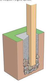
Whichever method is chosen, make regular checks with a spirit level, during the installation, to ensure that the posts remain vertical.
