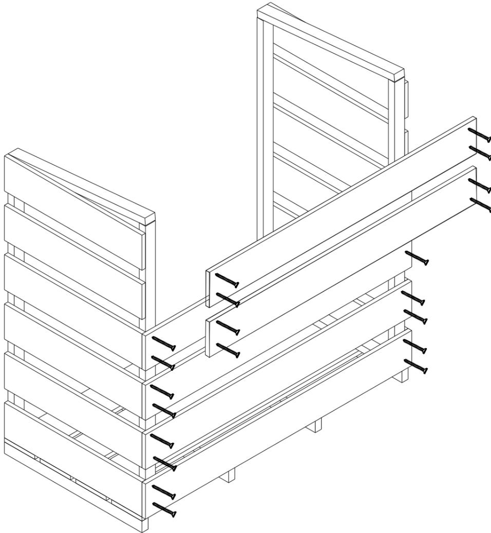
Once the sides are fixed to the floor attach the boards so that they are in line with the boards on the left and right hand side and secure using two 30mm screws at each end as shown
