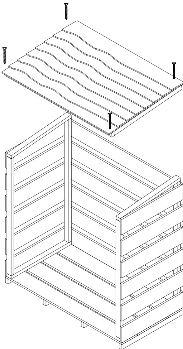
Place the log store roof on top of the structure so that the overhang is at the front.
