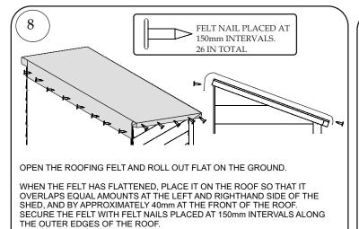
CUT AND FOLD FELT AT THE CORNERS AND SECURE FOLD WITH A FELT NAIL. FOLD FELT OVER THE BACK OF THE UNIT AS SHOWN ABOVE AND SECURE TO
